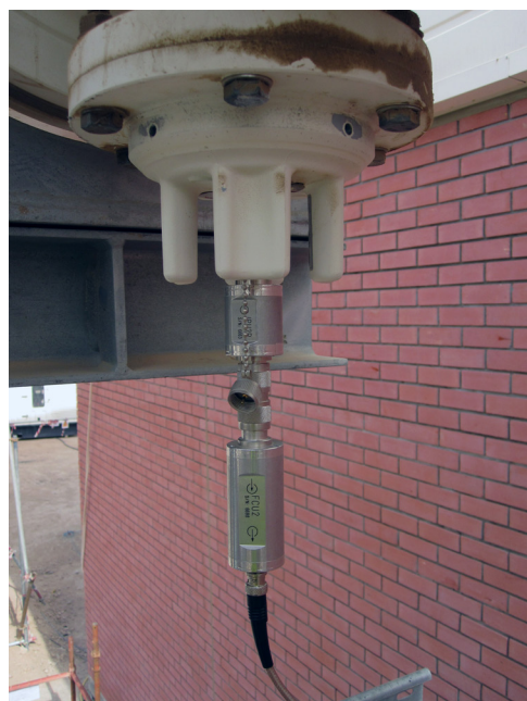
Figure 2: Vertical sensor, mounted with only an N-N adapter at an ABB outdoor GIS
