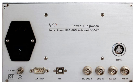
Figure 76: Back panel with MUX12 and TTL gating input
