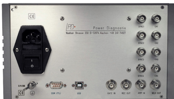
Figure 75: Back panel with MUX4 and RIV input
